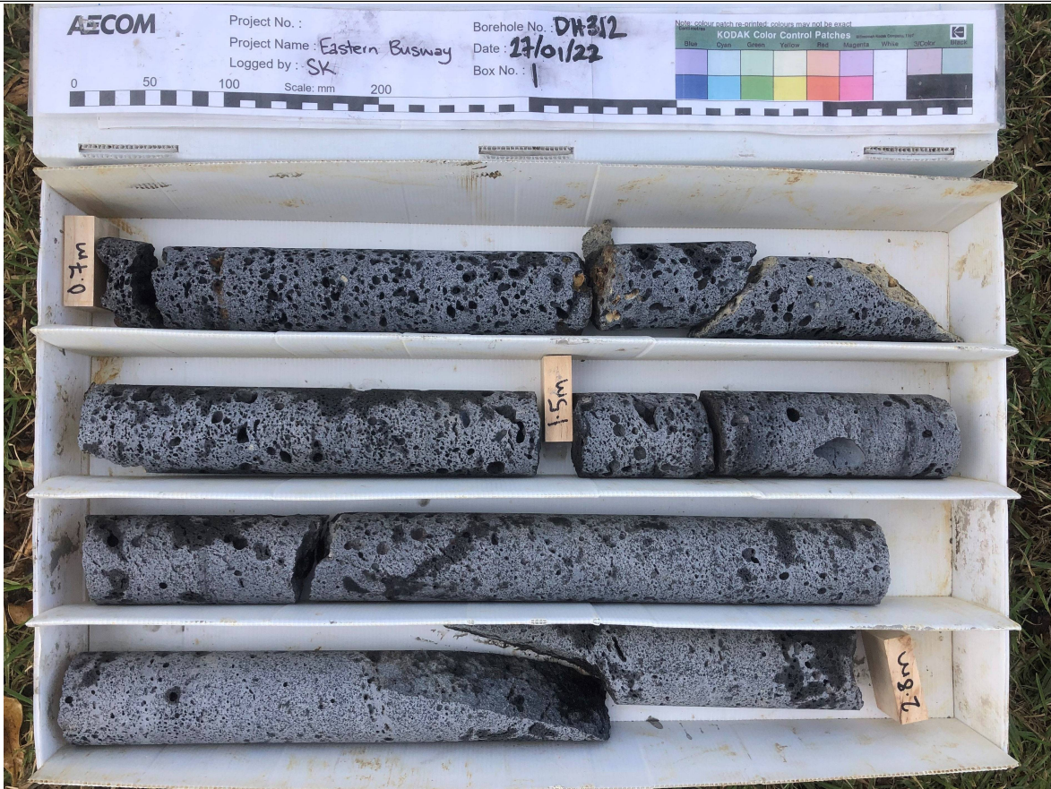
Box: 1 of 12 - Depth: 00.70m to 02.80m of 25.93m Date Drilled 27/01/2022 to 28/01/2022 - Date Photographed: 27/01/2022
