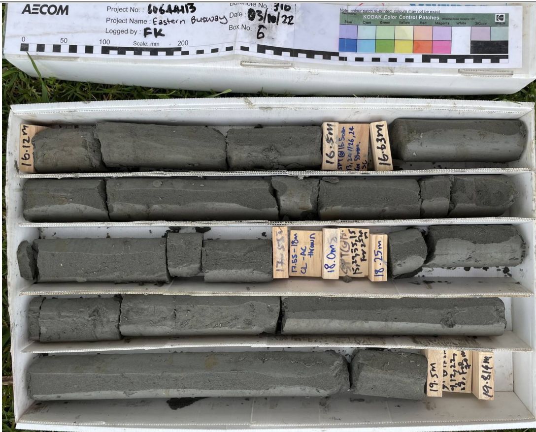
Box: 6 of 8 - Depth: DH310 16.12m - 19.814m of 25.00m Date Drilled 30/09/2022 to 10/03/2022 - Date Photographed: 3/10/2022
